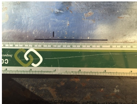
Figure 4 – Shoe front edge reference mark position
