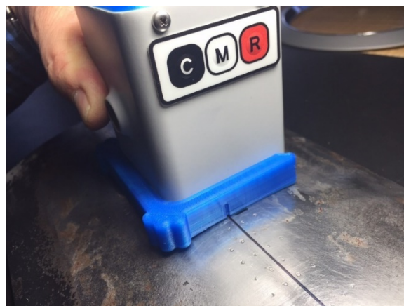
Figure 5 – Offset shoe position for Scanning with Ch-4
