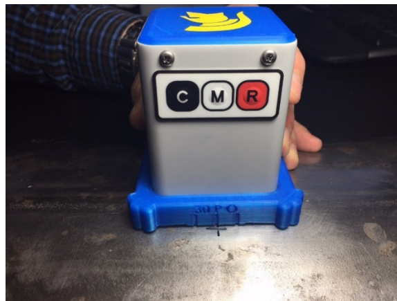
Figure 3 – Correct position of the offset shoe for Ch-0
